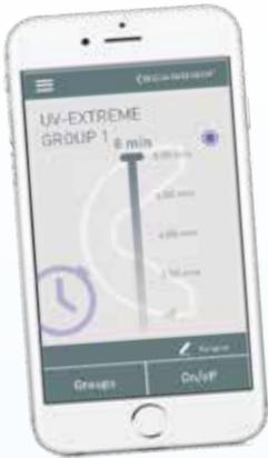
The built-in BLUETOOTH functionality makes it safe and easy to operate the lamp remotely, even in groups of up to 4 units simultaneously. Using the APP provides safe activation from a distance to avoid being physically close to the UV curing process.
